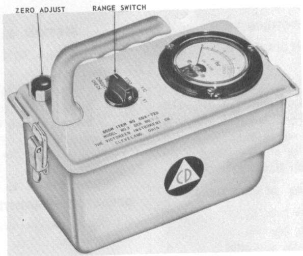
Figure 1. View of CD V-720, Showing Operating Controls
