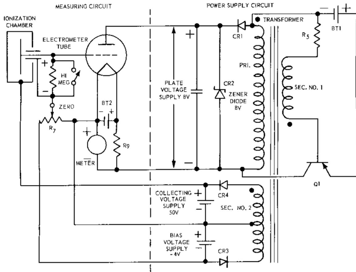
Figure 3. Simplified Schematic Circuit Diagram
