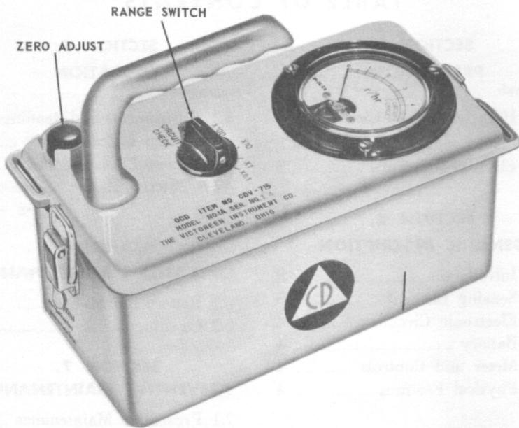
Figure 1. View of CD V-715, Showing Operating Controls
