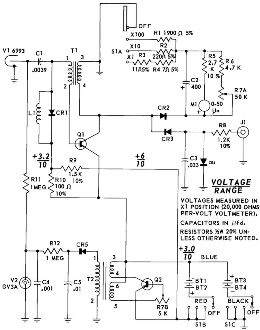
Figure 3. CD V-700, Model No. 6, Schematic Circuit Diagram
